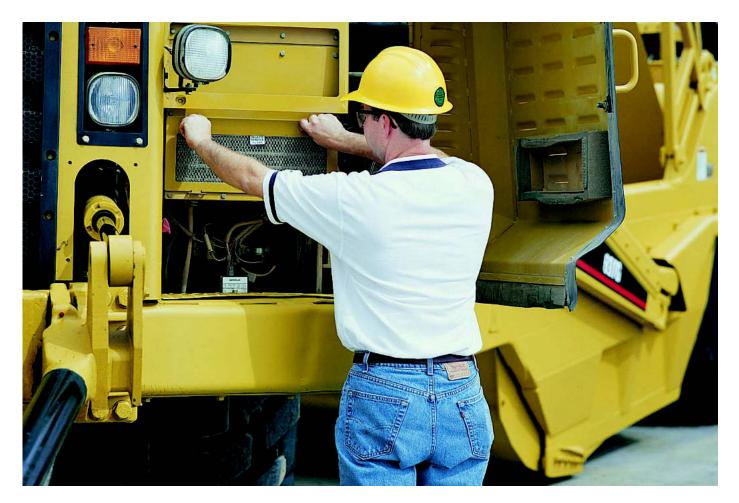
**Service Points.** Service points for the engine are grouped on the right-hand-side for easy access.
