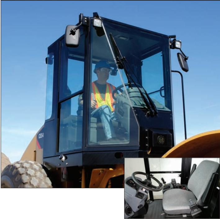
**Cab.** The cab provides a spacious and comfortable work environment that includes large windows, more interior room with storage areas, a cup holder, better ergonomics and low noise levels.
