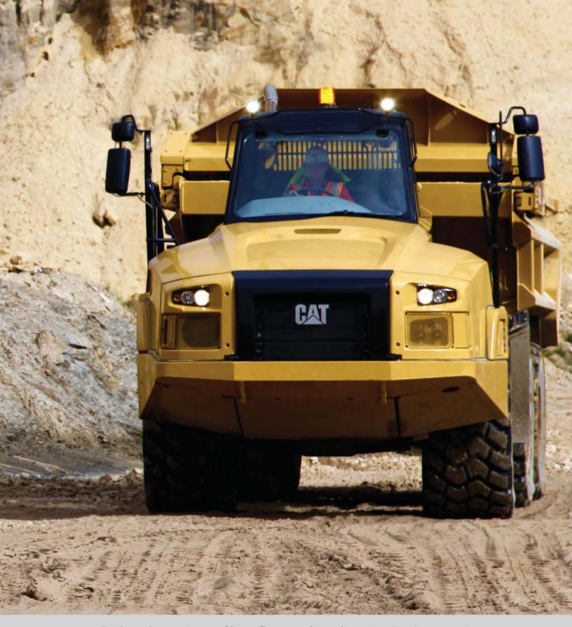
The Cat 730C2  $_{EJ}$ , with a 16.9  $_{m^3}$  (22.1  $_{yd^3}$ ) 28 tonnes (31 tons) capacity, offers demonstrated reliability and durability, high performance and productivity, superior operator comfort and lower operating costs.
