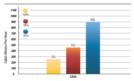
% Compaction of Standard Proctor 150 mm Crushed Limestone Base Results are similar for padfoot drum. Results may vary for different applications.
