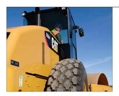
**Visibility.** The line of sight to the tire edges and rear of machine is exceptional. Operator can see obstacles measuring 1 meter high located 1 meter to the rear of the machine. Excellent visibility increases productivity when working near obstructions or maneuvering around the job site.
