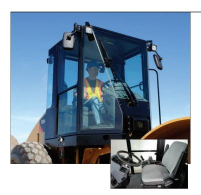
**Cab.** The cab provides a spacious and comfortable work environment that includes large windows, more interior room with storage areas, a cup holder, better ergonomics and low noise levels.
