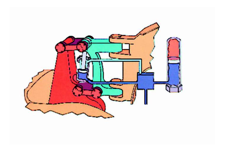
**Cushion Hitch.** Electrically actuated hydraulic damper absorbs haul road shocks for increased operator comfort.
