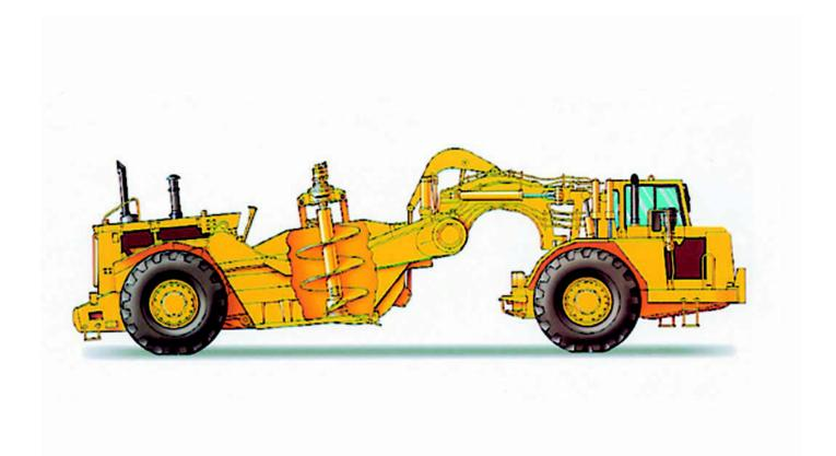
Material Application. Work alone capability with a wide material appetite ranging from overburden to laminated rock. Conditions material which promotes compaction in the fill and significantly reduces dust during loading.
